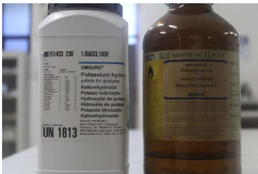
Figure 18. Diethyl Ether is a commonly peroxide forming compound. Adding KOH is recommended when storing ether for long time period (to form insoluble peroxide salt)
